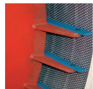
Rotor with beater ledges Conidur screen for fine milling
