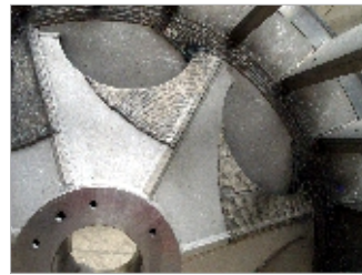
Wear Protection Rotor Hard-facing with special welding material for long life protection.
