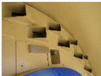
Air Guiding Nozzles The built-in fan supports the flake discharge from the knife ring top.
