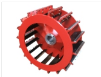
Rotor Long life wear protection by protecting the main body, shovel protection plate overlapping the blades.
